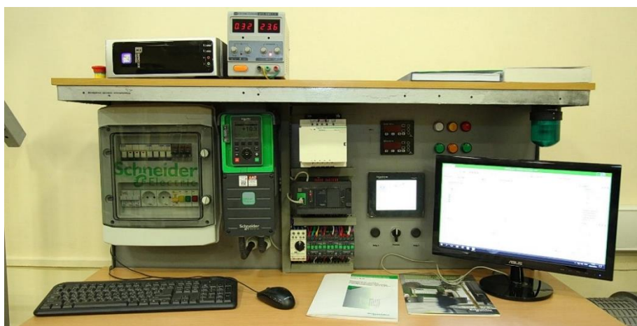
Figure 4: Laboratory stand for the study of a controlled induction electric drive
