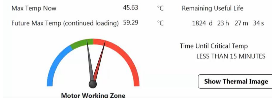
Figure 8: Digital panel of the current thermal state of the motor
