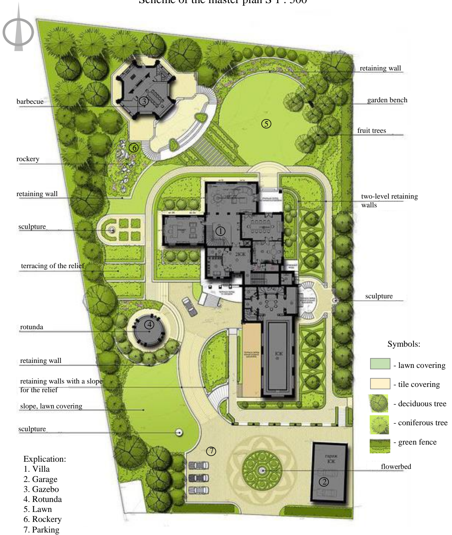
Figure D.2 – Example of design scheme of the master plan of a modern residential building (on the example of a villa in a natural environment)
