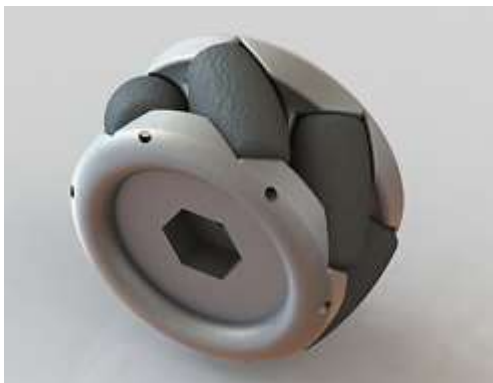
Fig. 1. 3D model of the Mecanum wheel
