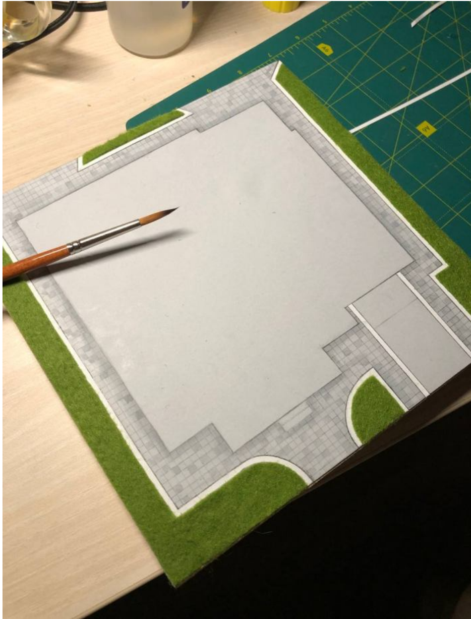
Figure 18 – Creating an imitation (paving tiles)
