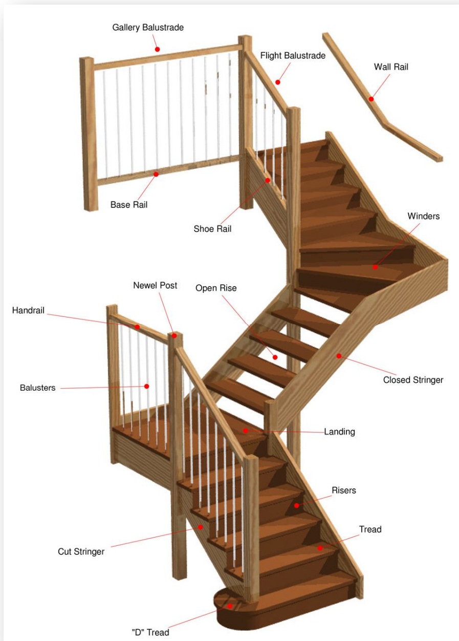
Figure 3.15 – Structure of stairs
