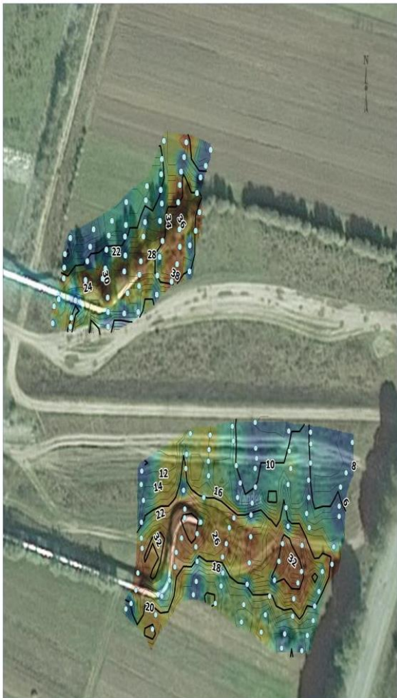
Fig. 2. Results of stress intensity of NPEMF gas pipeline Union and UPU.
