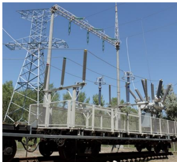
Fig.1. Mobile TS «Kremenchuk traction» of the regional branch «Pivdenna zaliznytsia» (Southern railways) of the Corporation «Ukrzaliznytsia» (Ukrainian railways)
