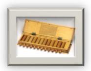
As the necessity demanded, scientist started inventing better calculating device. In thus process John Napier's of Scotland invented a calculating device, in the year 1617 called the Napier Bones. In the device, Napier's used the bone rods of the counting purpose where some no. is printed on these rods. These rods that one can do
