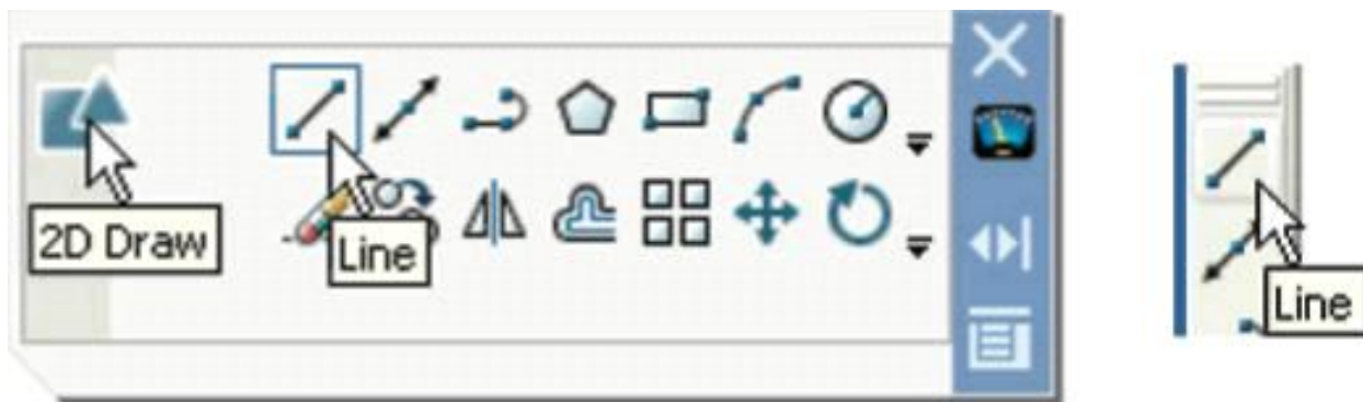
Figure 3.1 – Draw control panel
