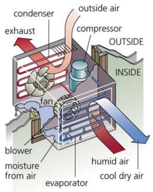
An air conditioner employs the same operating principles and basic components as your home refrigerator. Refrigerators use energy (usually electricity) to transfer heat from the cool interior of the refrigerator to the relatively warm surroundings of your home; likewise, an air conditioner uses energy to transfer heat from the interior of your home to the relatively warm outside environment.
